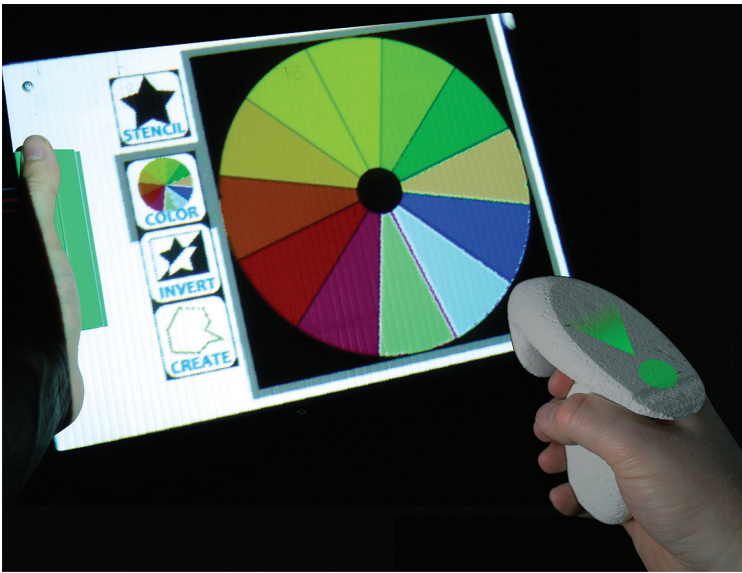
Figure 3. A physical-virtual-tool user interface for an airbrushing application. The user holds the stencil tool in his or her left hand. The system projects the controls onto the device, indicating the current mode and available modes. The airbrush tool, held in the right hand, has the spray angle, paint color, and brush type projected onto it.
