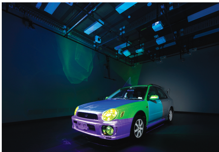
Figure 1. Spatial augmented reality (SAR) can change the appearance of large artifacts and can be viewed from all angles. In this case, the SAR system is projecting a wireframe and test textures to confirm the projector alignment.
