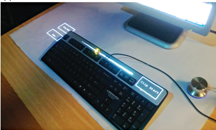
Figure 4. Two examples of ad hoc controls, in which the wooden cube is the handle for slider interaction. (a) Video-editing controls on their own. (b) The same controls supplementing the existing standard controls.
